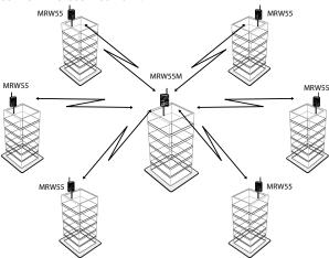
The MRW55 / MRV55M includes two antennas and operates in two bands, 2.4Ghz and 5 Ghz, making it ideal for configurations that need simultaneous Access-Point and Wireless Bridge connectivity.
